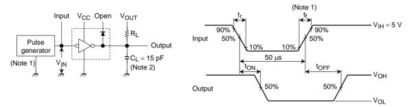
Note 1: Pulse Width 50  $\mu s,$  Duty Cycle 10% Output Impedance 50  $\Omega,$   $t_{f}$   $\leq$  5 ns,  $t_{f}$   $\leq$  10 ns
