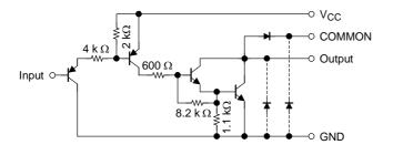
Note: The input and output parasitic diodes cannot be used as clamp diodes.
